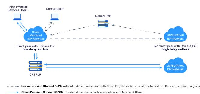
The chart below shows how the solution works:
